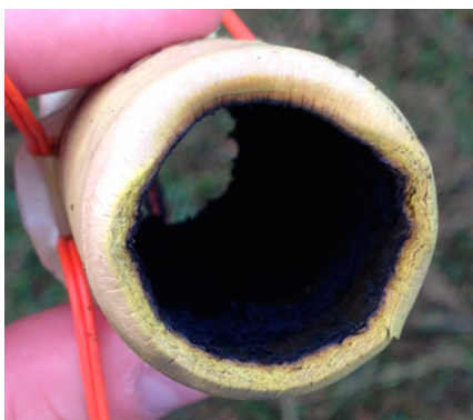
Figure 3. Candle image, postburn; note absence of top protector disc and parachute anchor.
